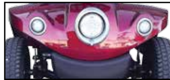
LED lighting system.
